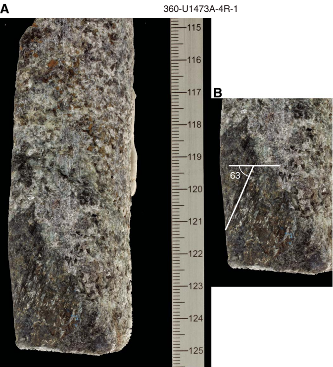
Figure F137. A. Fracture surface with slickenlines on olivine gabbro. B. Annotated image of the slickenlines with rake of 63° from y in the CRF.
