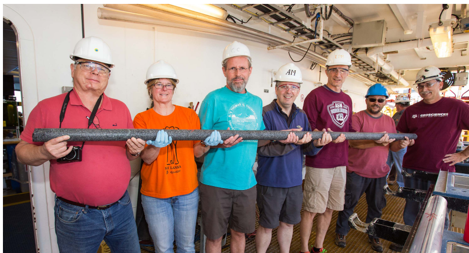
Figure F10. Longest piece (2.85 m) of rock recovered during Runs 17 through 21 (third coring episode; 519.2–789.2 m DSF), which yielded the originally expected excellent recovery (also see Figure F2B) with several unusually long pieces of rock recovered, Hole U1473A.
