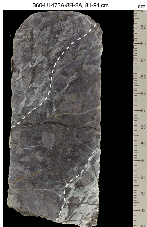
Figure F121. Mylonitic shear zone along contact between an oxide gabbro (upper) and olivine gabbro (lower). This is part of two 10 m thick mylonitic zones between 200 and 220 m CCSF. The mylonite (right side) is in contact with a moderately deformed porphyroclastic rock (left) (white dashed line). A thin ultramylonite layer defines the contact with the mylonite-porphyroclastic rock (yellow dashed line).
