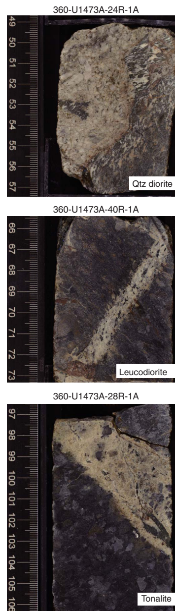
Figure F38. Quartz (Qtz) diorite, leucodiorite, and tonalite, Hole U1473A.
