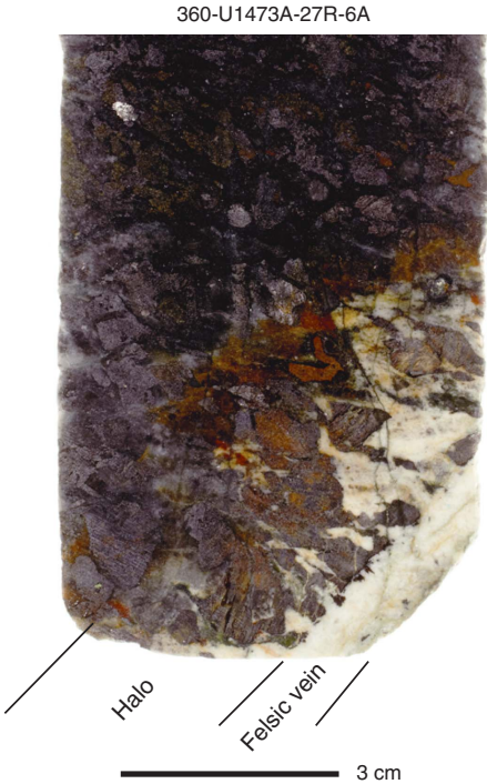
Figure F40. Felsic patch in gabbro, Hole U1473A. Felsic veins seem to infiltrate into the preexisting gabbro (red broken arrows).
