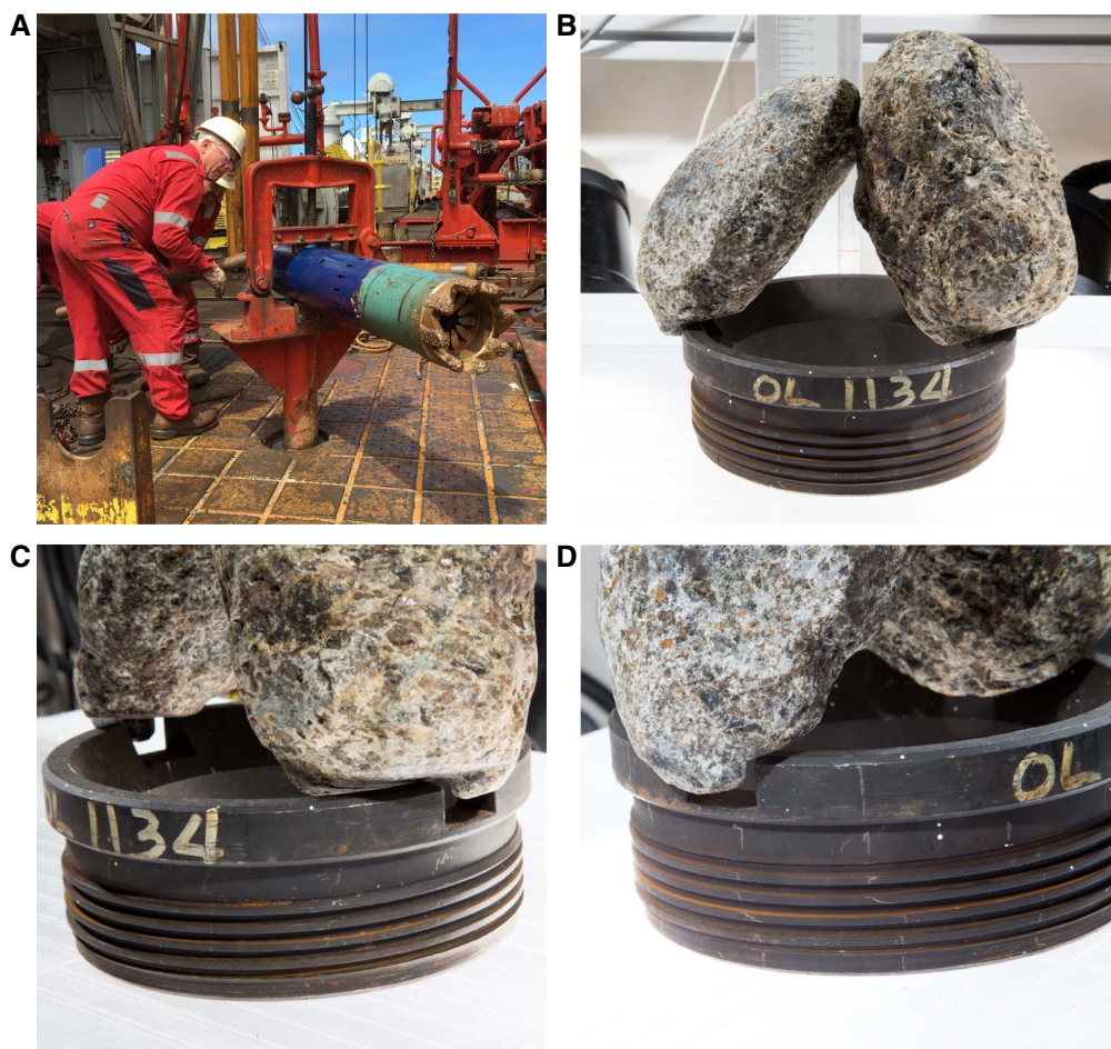
Figure F11. A. Attempts at fishing MBR retainer sleeve lost at bottom of Hole U1473A during logging operations (BHA Run 21) with RCJB Runs 22 and 24 were not successful. B–D. However, BHA Run 24 recovered two gabbro cobbles with tool marks that perfectly fit a spare retainer sleeve on board, which proved the presence of the sleeve at bottom of hole and indicated recovering (or milling) the sleeve is feasible.
