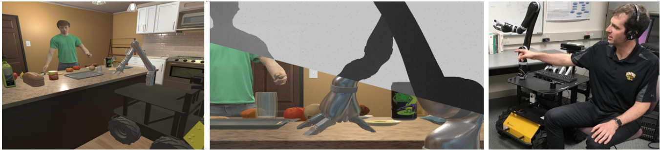
Figure 1: Our proposed Sim2Real human participant study. Left: a participant trains a robot on a grounded language task in virtual reality. Middle: the simulated robot percepts. Right: the learned model is tested on the physical robot.
