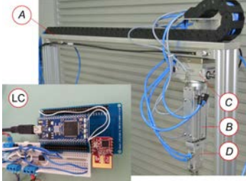
Fig. 7. Case study 1. A photograph of pneumatic manipulator with three degrees of freedom (A—translation; C—rotation; and B—translation) and gripper D; LC is MCU based with IEEE 802.15.4 compatible transceivers.
