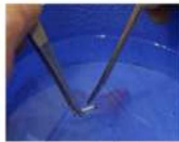
Insert the rotor into the microcentrifuge tube cap forward. We recommend pushing the rotor in rather than grabbing it with the tweezers.
