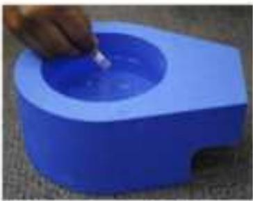
Slide the rotor into the liquid nitrogen bath.
