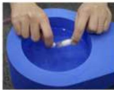
Approach the surface of the liquid nitrogen and unscrew the top of the cryovial.
