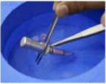
Lift the sample catcher and the tube as soon as the sample catcher is in the microcentrifuge tube.
