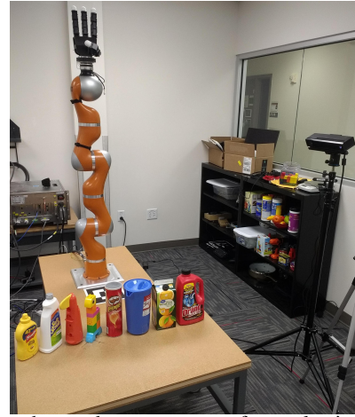
Fig. 5: Our robot and camera setup for evaluating grasping in the real world with a KUKA LBR4 robot with Allegro end-effector. The objects are labeled from left to right as mustard , soft-scrub , airplane-toy , Lego , pringles , pitcher , juice-box , and max-gel respectively.
