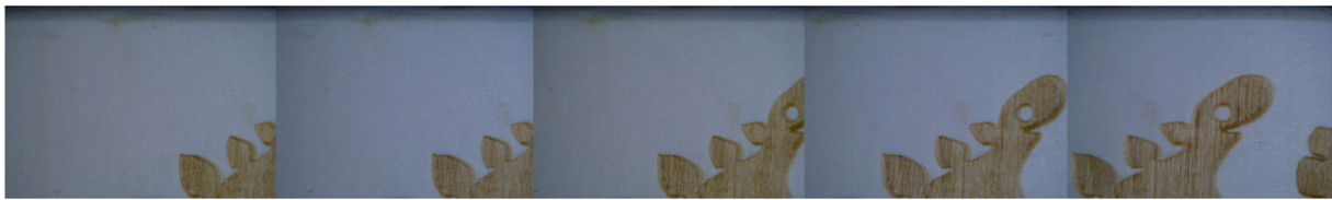
Fig. 14. End mill tool phase-shifting raw image from location 1~5.
