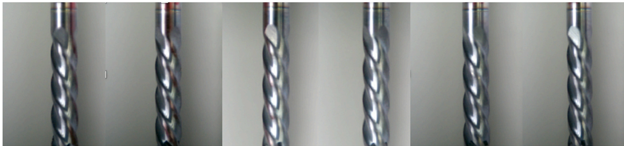
Fig. 11. End mill tool phase-shifting raw image from location 1~6.
