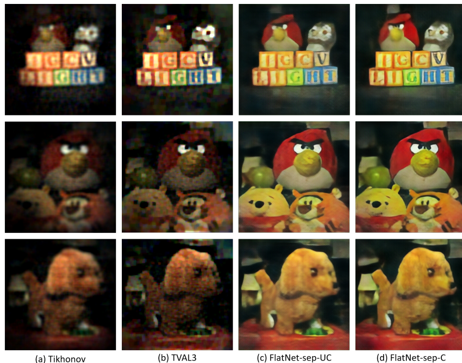
Fig. 5. Direct Captured Reconstructions for FlatCam: a) Details in the border and darker regions are lost in the Tikhonov regularized reconstructions. b) TVAL3 reconstructs the border but is unable to restore the sharpness. The proposed end-to-end models for both c) random and d) transpose initializations produce the best reconstructions. These methods are robust to noise and does not contain any regularization parameters.
