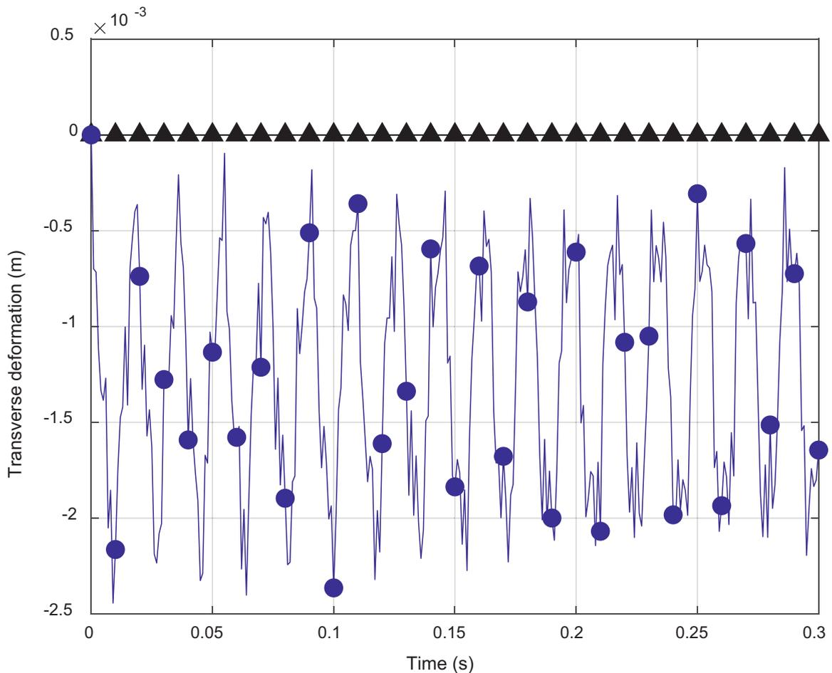
Fig. 2. End-effector forward-dynamics transverse deformation (—▲— With deformation actuation, —●— Without deformation actuation).
