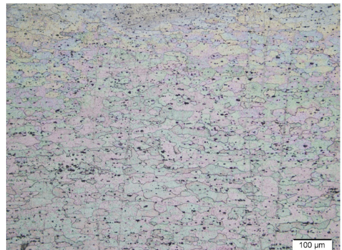
Fig. 1. Optical micrograph of the grain structure in the as received Al-6061 alloy.
