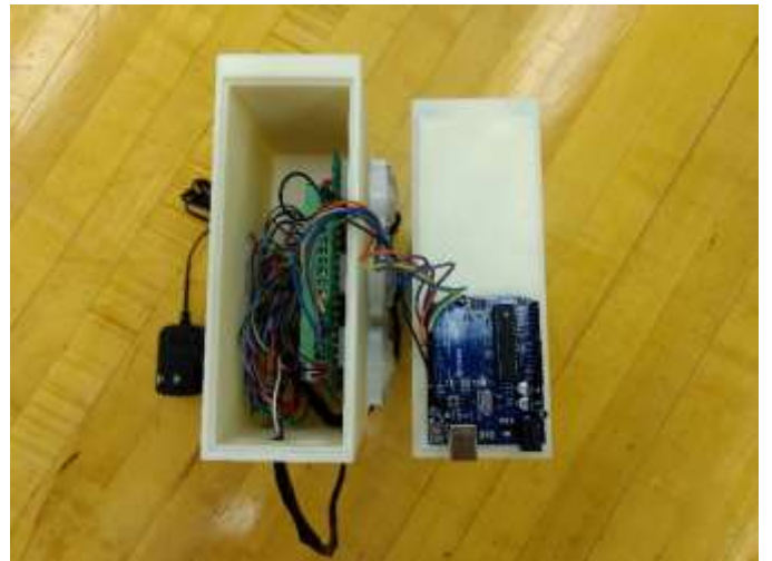
Fig. 10. Arduino and Relay Integration
