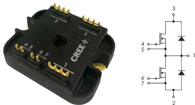
Fig. 1. A picture of the custom 1200-V SiC half-bridge module used in this work and its schematic.
