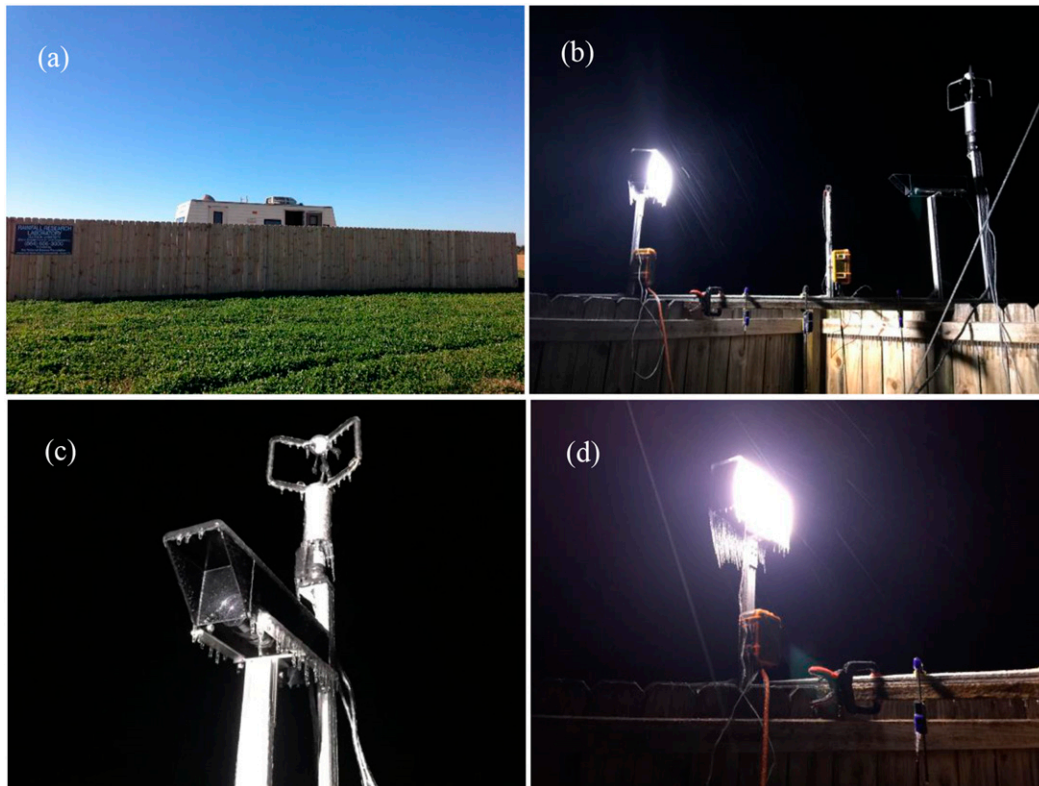
FIG. 1. Photographs showing (a) the field site, (b) the HOD installed over the wooden fences at 2 m above the ground surface, (c) the icicle formations on the HOD's high-speed camera enclosure and the ultrasonic anemometer, and (d) the light source during the freezing rainfall events.
