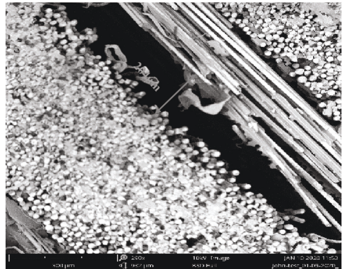
Fig. 7. SEM image of GFRP composite laminate after impact, with severe delamination.
