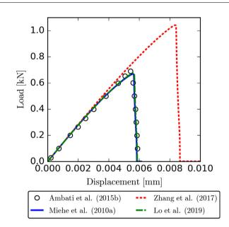
**Fig. B.2.** Load-displacement curves for single edge notched tension test. The solid and dashed lines depict the numerical results obtained from phase field model based on the corresponding strain energy decomposition schemes. The black circular maker represents the benchmark solution digitized from Figure 9 of [34].
