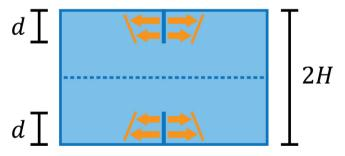
**Fig. C.1.** Double edge cracks through finite slabs with H in width and d in crack length. The yellow arrows indicate applied loading on the crack surface that leads to crack opening. The dashed line of symmetry represents the free slip surface at the base of the glacier.
