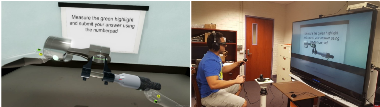
Figure 1: Left: Bimanual interaction in a virtual precision metrology training simulation as seen in a head-mounted display (HMD) presentation condition. Right: Viewing and spatially interacting with objects in a stereoscopic large-screen immersive display (LSID) presentation condition.
