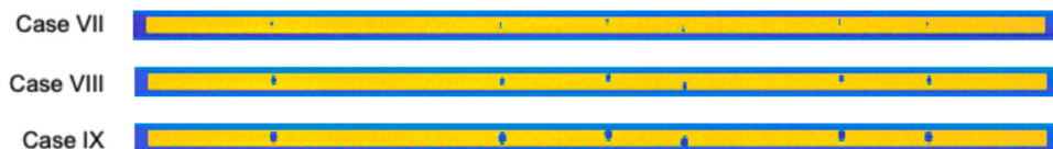
Fig. 15. Simulated thin-walls with different pore sizes but same number of pores. Case VII: diameter 2 pixels, case VIII: diameter 4 pixels, case VI: diameter 6 pixels.
