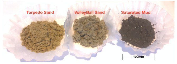
Fig. 3: The three soils used for the experiments. 0.125 cubic meters of each soil type was placed in three plastic bins for the drop experiments.
