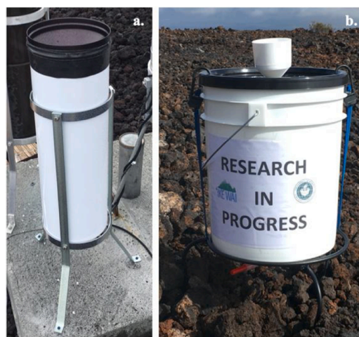
Fig. 2. (a) A NovaLynx Rain and Snow Gauge, deployed at the Mauna Loa Observatory. (b) A bucket-style rain collector, deployed at Humu'ula.
