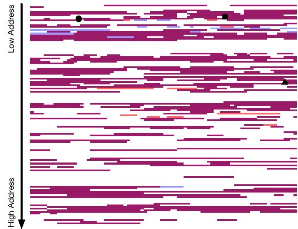
Figure 4: Bitmap of instruction traces collected on Laelaps and the real device. Purple color represents overlapped trace segments. ● marks the end of device setup (phase 1). ■ marks the end of base system setup (phase 2). ▲ marks the end of RTOS initialization and the start of the first task (phase 3).
