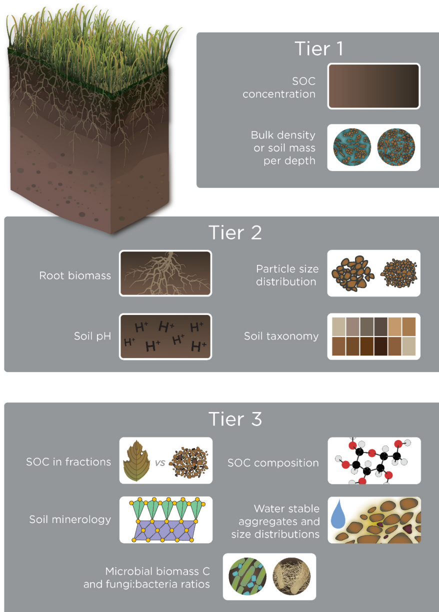
FIG. 1. Summary descriptions of soil features and properties to quantify or characterize to gain an understanding of soil organic C (SOC) pool sizes and mechanisms of its formation, retention, and losses. Features are arranged into three tiers representing a gradient of complexity, from the simplest (Tier 1) to those requiring greater investigator investment (Tiers 2 and 3). For all tiers, site-level data such as latitude and longitude, landscape position, and vegetation cover and type should be collected to contextualize SOC data.
