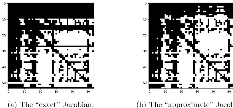
Figure 4: A graphical representation of the sparsity pattern of the chemical kinetic Jacobian generated by pyJac for GRI-Mech 3.0. Black squares indicate a non-zero Jacobian entry, while white square correspond to an empty entry. The numbers indicate the index of the entry in the state vector.
