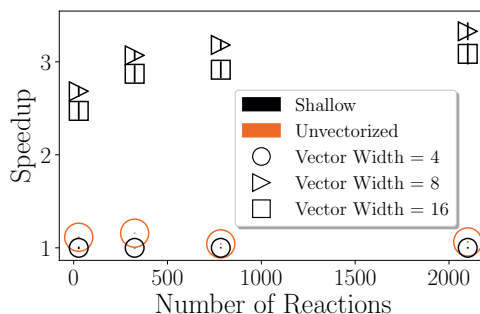
(d) The effect of vector-width on “C”-ordered shallow-vectorized Intel OpenCL source-term evaluations on the avx2 CPU.
