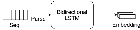
Fig. 7. Proof Script Encoder. The proof script encoder’s input is a sequence of proof script tokens, which it parses and then uses to generate an embedding using a Bidirectional LSTM.
