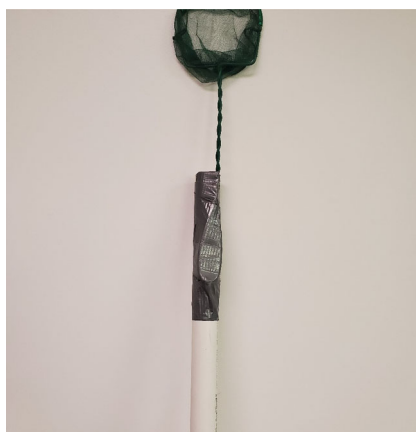
Figure 2. An example of the net used to sample larval silver carp and other fishes in shallow water habitats.
