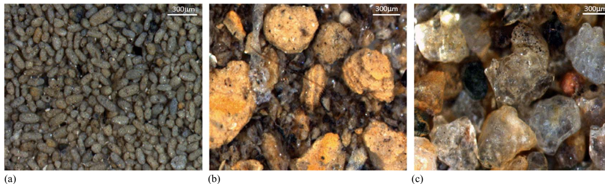
Fig. 4. Images collected under 30× magnification of nondispersed and nonsonicated sediment retained on 63 µm mesh: (a) Core 12 1–2 cm; (b) Core 14 3–4 cm; and (c) Core 2 3–4 cm.
