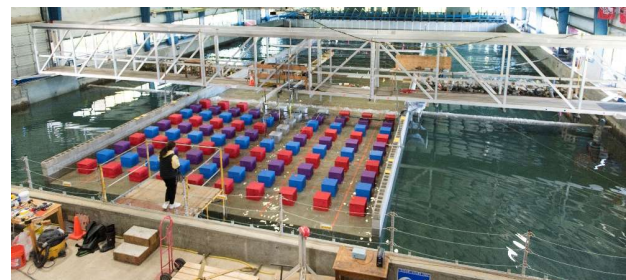
Figure 2 - Overview of the developed barrier island in the DWB during a test execution. In the foreground, the coastal community represented by 100 buildings. On both sides, the return flow sections, pumps and wave absorbers.
