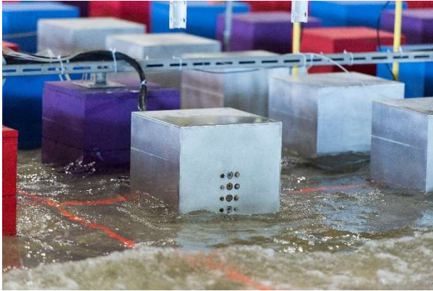
Figure 3 - Detail of the instrumented buildings (identified by the silver boxes) during an irregular wave test. Two buildings were fitted with a vertical array of pressure gauges (shown at the center of the image), five with in-line load cells (shown on the background of the image), and one with a submersible multi-axial load cell (not shown).
