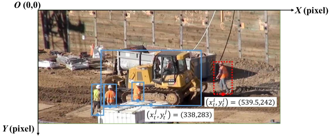
Figure 3 Pixel coordinates of construction entities (Entity i is the target, j is its nearest neighbor)
