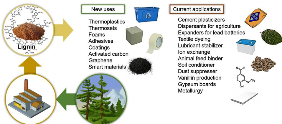
**Fig. 2.** Lignin-based materials in the current market and for future applications.
