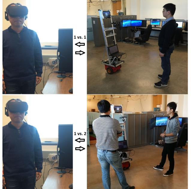
**Fig. 4** The application scenario of an immersive VR-based telepresence system (top images: 1 vs. 1 conversation. Bottom images: 1 vs. 2 conversation)
