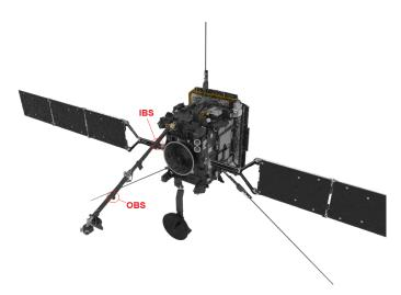
Fig. 4. Solar Orbiter spacecraft with MAG sensors marked.
