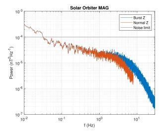
**Fig. 7.** Power spectra of normal and burst-mode data from the Solar Orbiter magnetometer flight model outboard sensor, operating in the most sensitive range. A single axis is shown. The 10 pT Hz<sup>-1/2</sup> at 1 Hz noise requirement is marked for reference.
