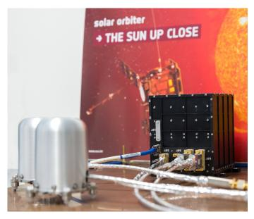
Fig. 3. Solar Orbiter flight hardware magnetometer sensors and electronics box.
