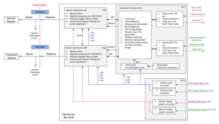
Fig. 5. Solar Orbiter magnetometer functional diagram.
