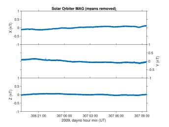
Fig. 8. Magnetometer data (means removed) taken within a magnetic shielding can at Imperial College London. Drifts over the >12 h interval are typical of local variations rather than sensor offsets.
