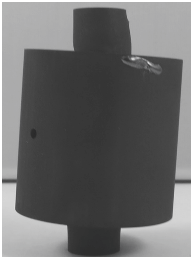
Fig. 2. Photograph of the deformed punches after the flash spark plasma sintering tests. (A colour version of this figure can be viewed online.)
