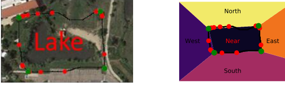
Fig. 2: Left: Convex hull vertices (red), reduced to 4 points with sequential hull reduction (green). Right: Softmax function and labels resulting from reduced points.
