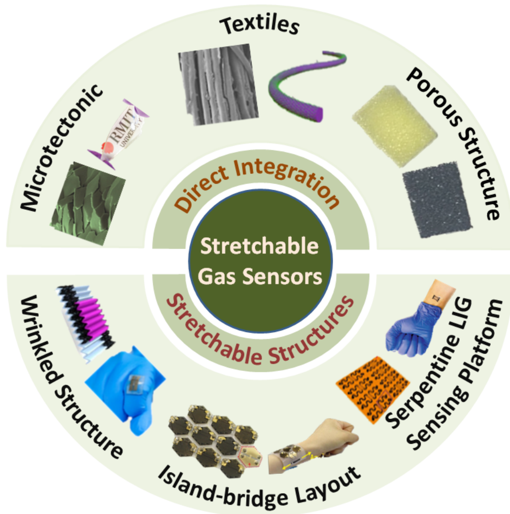
Figure 1 | Stretchable gas sensors enabled by direct integration of gas-sensitive nanomaterials onto the stretchable substrate (template) or by the exploration of stretchable structures. The stretchable substrate template in the former can be thin films (with a microtectonic sensing layer), textiles, porous (fibrous) structures. Reprinted with permissions from Refs [68-70]. The commonly used stretchable structures in the latter include wrinkled surfaces, island-bridge layouts, strain isolation layers, or their combinations as in the stretchable laser-induced graphene (LIG) gas sensing platform. Reprinted with permissions from Refs [71-73].
