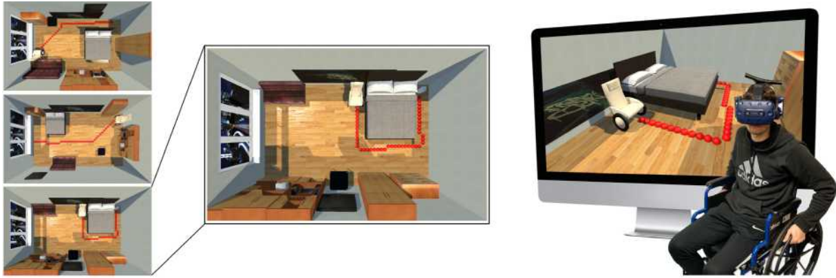
Figure 1: We have developed an optimization-based approach to automatically generate the scenarios (left) used for wheelchair training with different user-specified levels of difficulty. We test our generated scenario by developing a training program using VR trackers attached to the wheels of a stationary wheelchair to simulate motion in virtual space(right).
