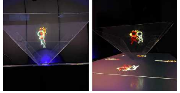
Figure 5. We used Pepper's ghost to illuminate images to the center of the hologram. The user could view the illuminate images from different views: front, back, and two rear views. Each view gives a different perspective.
