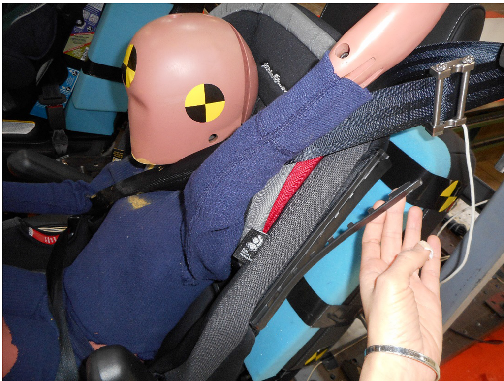
Broken track of booster shoulder belt guide
