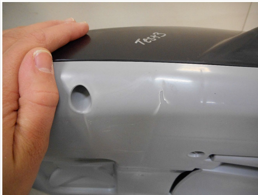
Evidence of bending and minor crack on RF CRS base.
