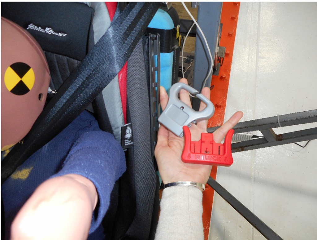
Broken booster shoulder belt guide.
