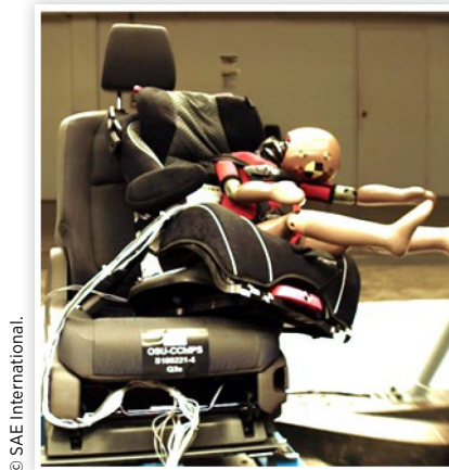
FIGURE 12 In all FF CRS conditions, the head of the Q3s translated past the CRS side wing. The image above shows the excursion of a control installation
