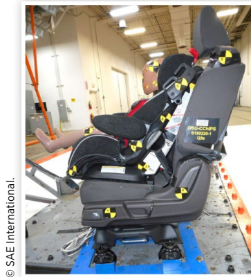
FIGURE 5 FF CRS with vehicle seat too acute
