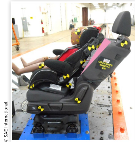
FIGURE 6 FF CRS with vehicle seat too obtuse
