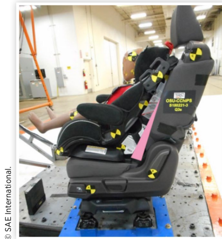
FIGURE 5 FF CRS with vehicle seat too acute
