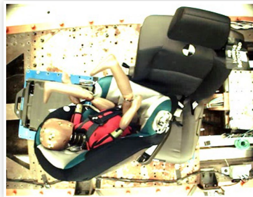
FIGURE 9 In all RF CRS conditions, the head of the Q3s rolled along the side wing and a torsional moment was produced on the neck. The image above shows an overhead view of a control installation
