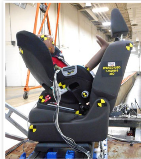
FIGURE 1 RF CRS control condition (good fit)
