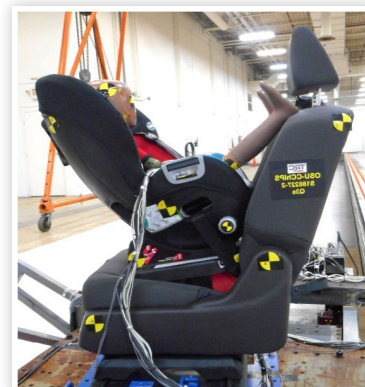
FIGURE 2 RF CRS pool noodle condition
