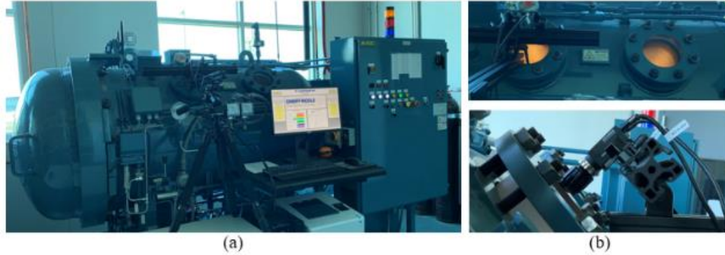
Fig. 1 (a) Autoclave with 3d DIC. (b) Autoclave viewports and DIC cameras
