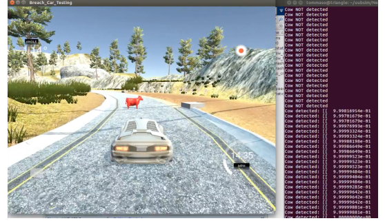
Fig. 6. Udacity simulator with a CNN-based AEBS in action.
