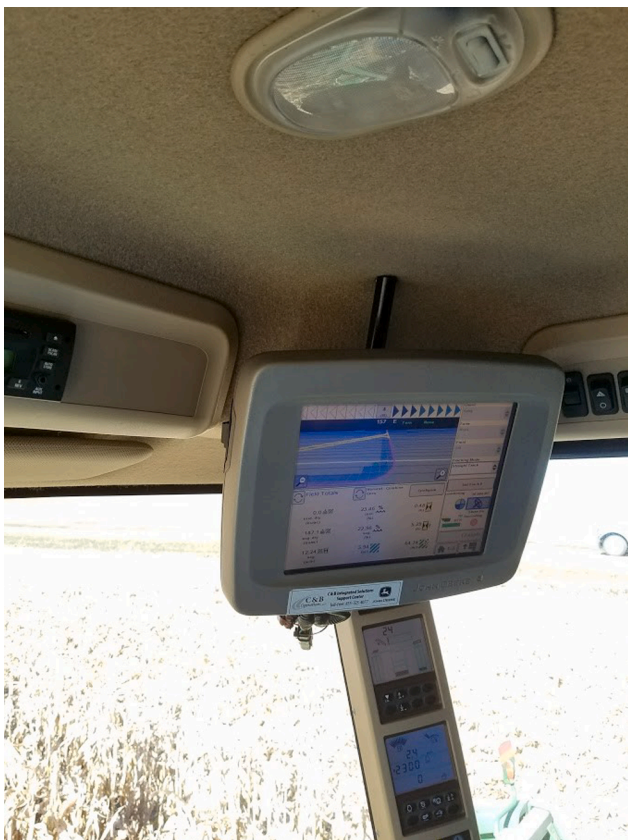
Fig. 1. Yield monitor being used by a farmer inside the cabin of a combine harvester (courtesy: John McMaine).
