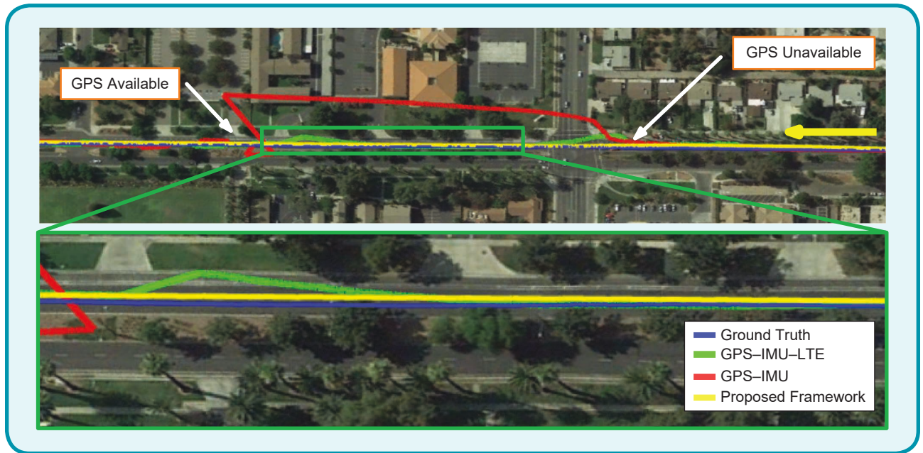
FIG 7 The vehicle's estimated trajectory from the GPS-IMU system versus the proposed framework when GPS signals become unavailable and then available. As can be seen, the GPS-IMU solution drifts in the absence of GPS signals. In contrast, the proposed framework does not exhibit such drift, as cellular signals are used as an aiding source to the IMU. (Source: Google Earth.)
