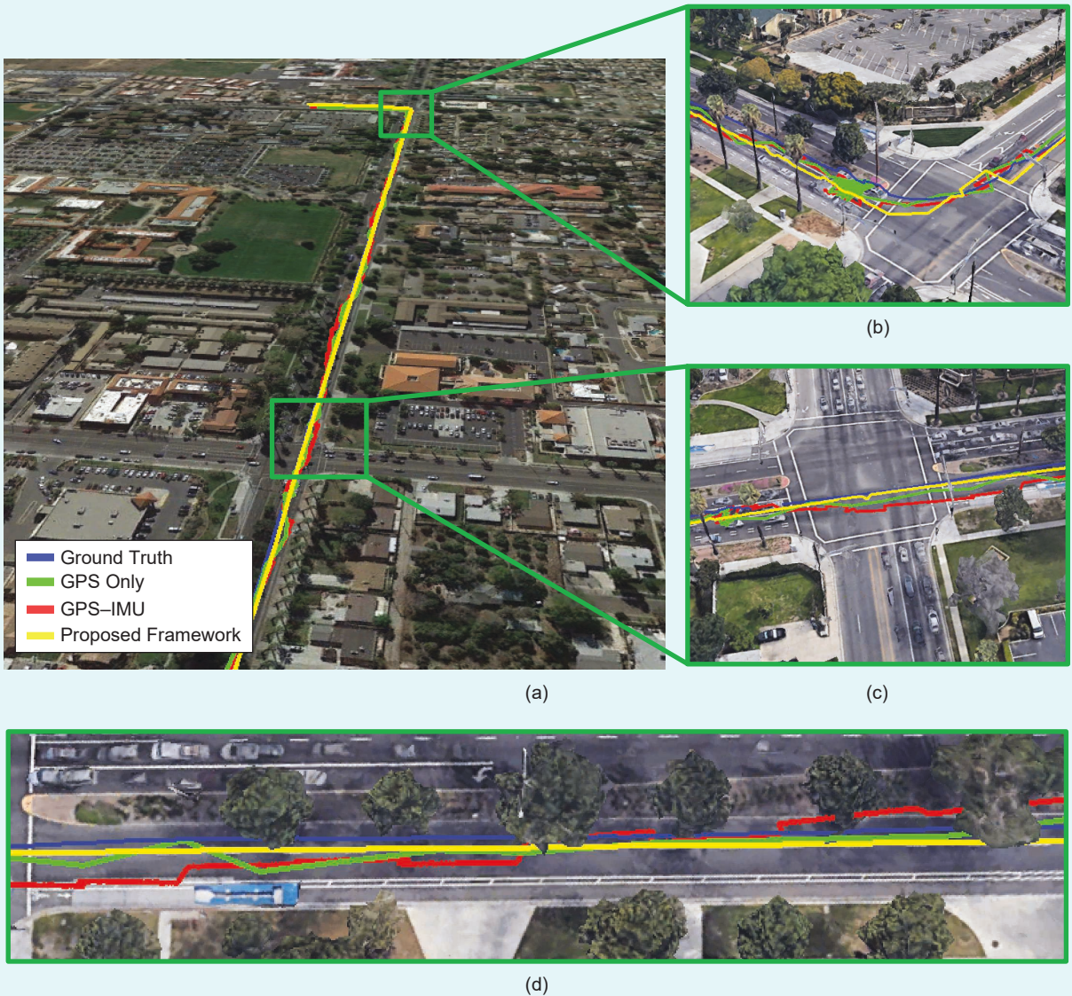
FIG 6 (a)–(d) The experimental results in an urban environment. The vehicle's estimated trajectory with our proposed framework is compared against the estimated trajectory with GPS-only and GPS-IMU systems. The ground truth was obtained with an expensive GPS-IMU system with RTK. Experimental results indicate a 2.8-m RMSE for the proposed approach. (a) The overall trajectory. (b) A turn segment at a crossroad. (c) A straight segment at a crossroad. (d) A straight segment surrounded by tall trees. (Source: Google Earth.)
