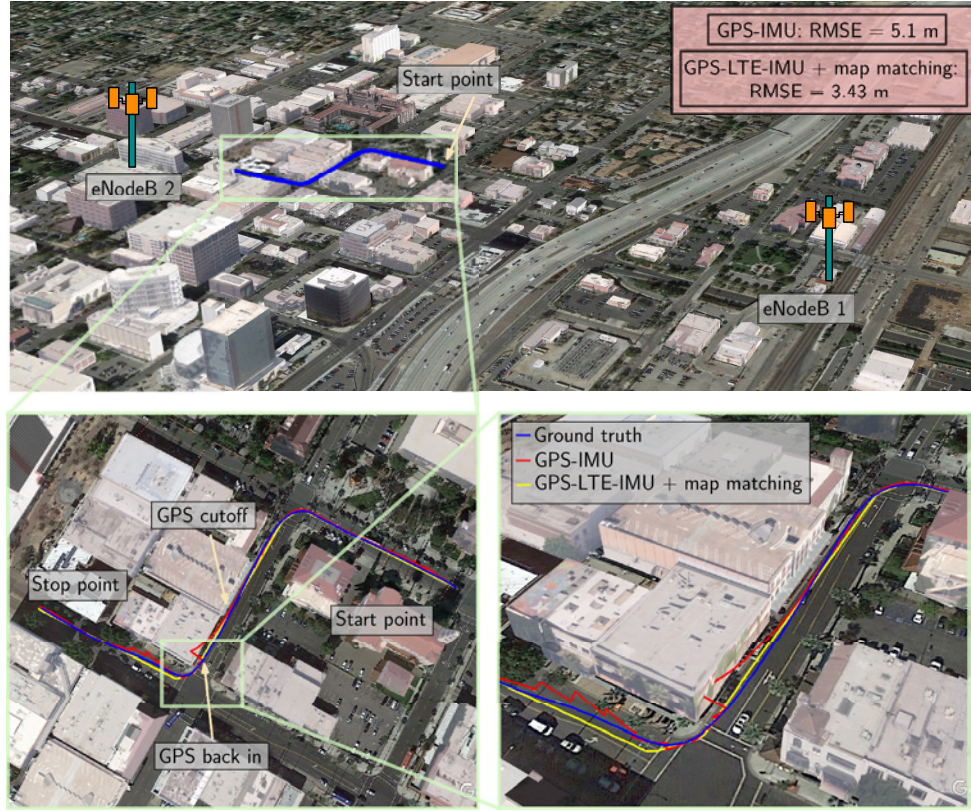
Fig. 4. Ground vehicle navigation with an integrated navigation system, which used GPS and LTE SOPs along with an IMU and map matching in a deep urban environment in downtown Riverside, California, USA. The figure shows the environmental layout, LTE eNodeBs' locations, traversed trajectory, and the different navigation solutions. Over a trajectory of 345 m, the GPS-LTE-IMU with map matching exhibited a position RMSE of 3.43 m compared to 5.1 m achieved using GPS-IMU only [63]. Map data: Google Earth.
