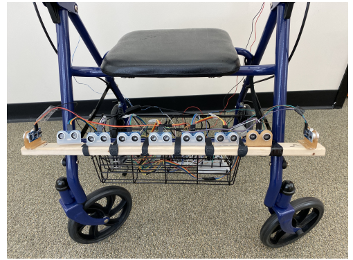
Fig. 1. The walker configured with ultrasonic sensors
