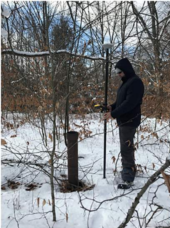
Fig. 15. Unplugged previously unknown well located with UAV-based magnetics. GNSS receiver staff is 2 m for reference.
