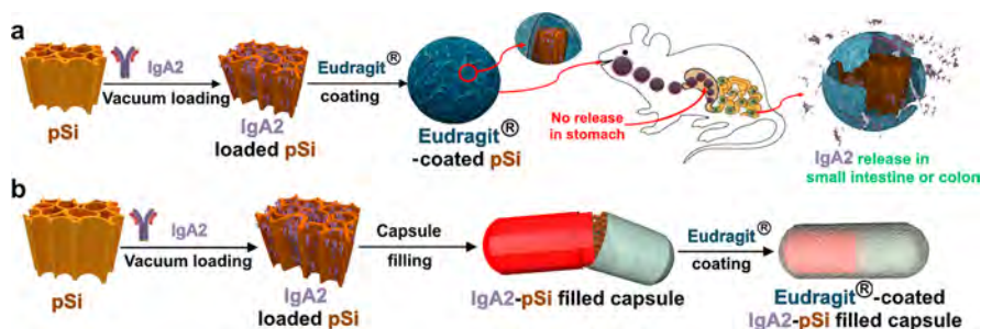
Scheme 1. (a) Schematic Illustrating the Preparation and the Proposed Fate of Polymer-Coated Porous Silicon (pSi) Nanoparticles for Oral Delivery of IgA2 a and (b) Schematic Illustrating the Preparation of IgA2-Loaded pSi Nanoparticles for Capsule-Based Delivery b
