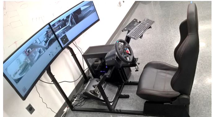
FIGURE 5. REMOTE CONTROL CONSOLE AND DRIVING CELL
