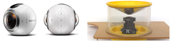
FIGURE 8. AN OFF-THE-SHELF DUAL-SENSOR 360-DEGREE CAMERA AND AN FPV-CAMERA + CONIC MIRROR SETUP
