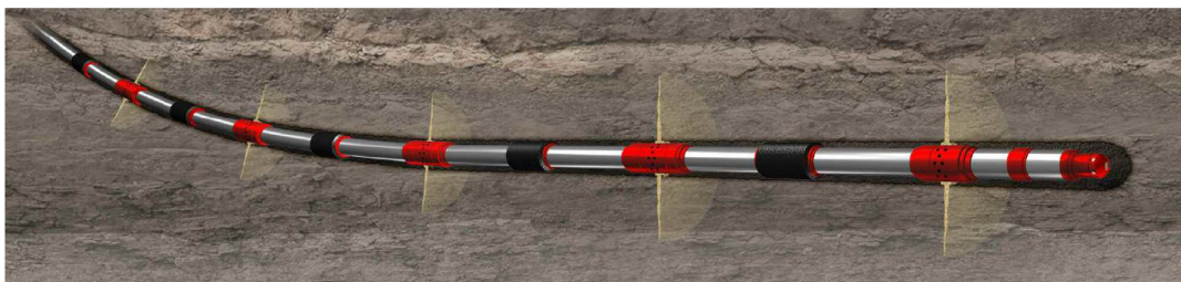
Figure 3: Illustration of multistage acid fracturing in a horizontal well [6]
