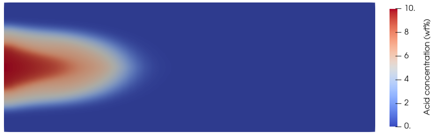
Figure 16: Acid concentration in vertical well acid fracturing treatments (pad is polymer)
