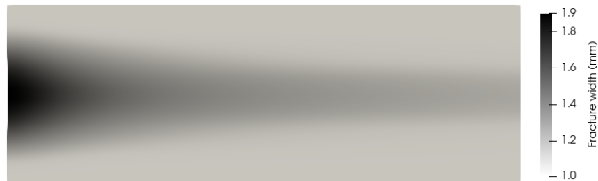
Figure 11: Field of fracture width in vertical well acid fracturing treatments (pad is polymer)
