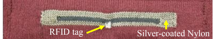
Fig. 1: Bellyband antenna [6]. The conductive part of the antenna is made from silver-coated nylon.
