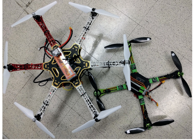
Fig. 3: UAVs used for collecting measurements. (Left) shows a DJI F550 Hexacopter, UAV 1 for short, and (Right) is a Turnigy SK450 Quadcopter powered by Multistar, UAV 2 for short. Top view is the one facing the horn antenna and is noted as 0° in the measurements section IV where it was then azimuthally rotated one complete cycle in 45° increments.
