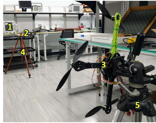
Fig. 4: RCS mmWave measurement setup. 1: KEYSIGHT 67 GHz PNA-X Network Analyzer N5247A, 2: 25 dBi standard horn antenna, 3: UAV 2 of Figure 3, 4: Fixed tripod, 5: Adjustable camera tripod.
