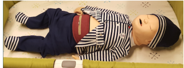
Fig. 1. A programmable mannequin Simbaby wearing the Bellyband about the abdomen. The Bellyband stretches and relaxes during respiratory activity, which is observed through changes in RF reflected from the knitted antenna on the Bellyband.
