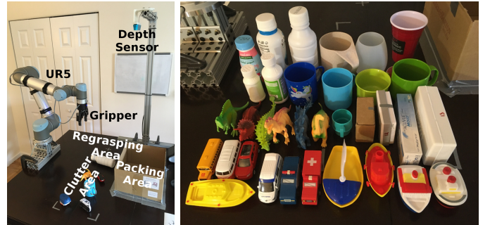
Fig. 4: Left . Environment includes a UR5 arm, a Robotiq 85 gripper, and a Structure depth sensor. Right . 34 same-category novel objects used for real-world packing experiments.
